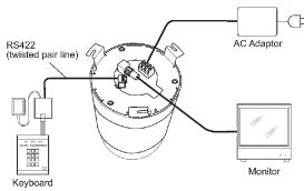
Make sure to connect to a power supply that allows for at least 35W consumption.
